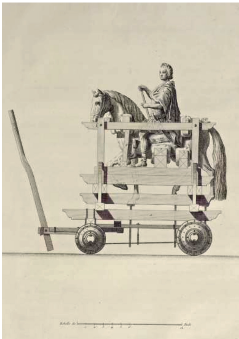
Statue moving Perrault technique
